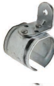
11-SLB Bracket Face mounted heavy duty bracket allows adjustment in spacing. Also acts as splice. Use with #11 slotted track.
